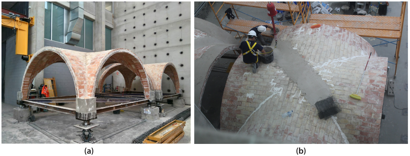
Figure 1: Experimental tests on timber masonry cross vaults (a) original/unreinforced specimen; (b) reinforced vault with TRM.
